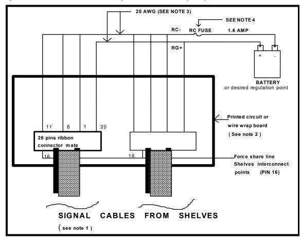
Figure 8 · No controller, remote sensing connection for a 26-pin signal connector shelf
